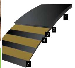
1. Top Cover: Made from super abrasion resistant natural Rubber. Tested to EN ISO 14890:2003 - Specification for rubber or plastic covered conveyor belts or textile construction for general use.
