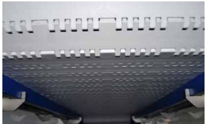
After the inclined section the belt runs via a radius horizontal where the Flight is de-activated and the belt becomes flat again.
