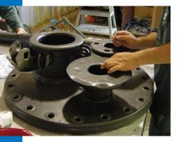
reinforced stocks. These compounds are formulated for services involving wet chlorine, strong acids at high operating temperatures, plating solutions and water conditioning equipment. All have a soft tie gum for maximum adhesion to steel.
